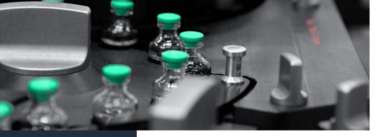
A 100 percent in-process control (IPC), which weighs each container before and after filling, makes sure that each previously approved vial contains the exact amount of active ingredient.
