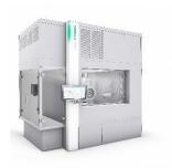
Versynta microBatch is a highly flexible fully automated production cell with a gloveless isolator, the smallest possible dimensions, and a complete batch-to-batch changeover of less than two hours.
