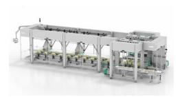
Syntegon's newest cartoner, Sigpack TTMD, combines core components of the TTM platform with one or more seamlessly integrated Delta robot cells – this allows flexible packaging of different products.
