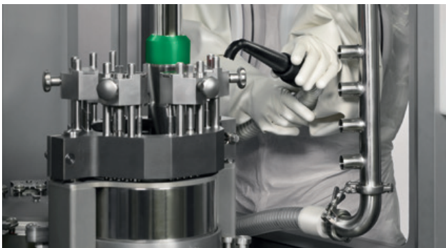
Pre-cleaning and flushing of the processing area
