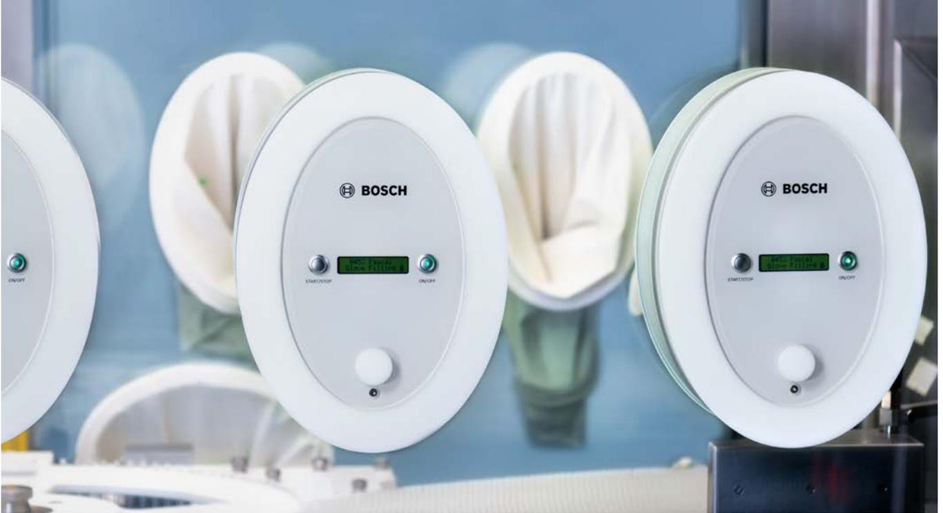
▲ Glove testing device in isolator execution
