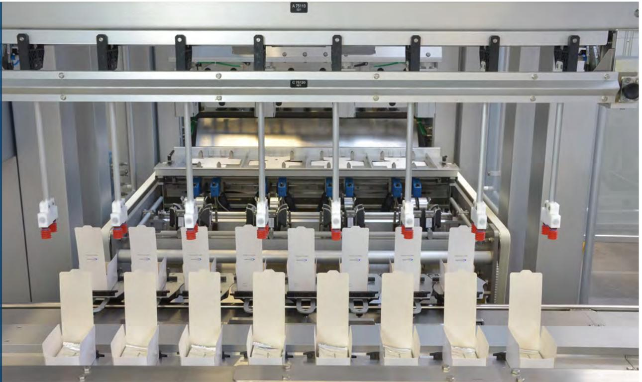
The bulk vial cards are first manually loaded into an intelligent feeding unit, which unscrambles and separates them equidistantly. It then aligns the individual vial cards before transferring them onto a conveyor. The intelligent feeding unit operates at adjustable speeds, with an output of up to 300 pieces per minute.
