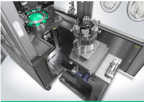
Fast product changeover by plug-in station
