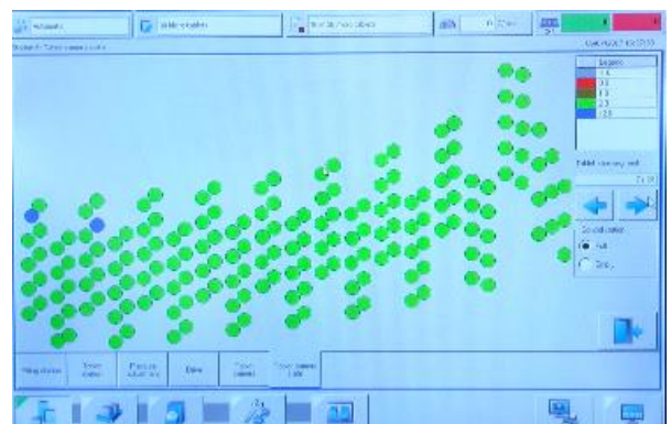
HMI with camera control result of 10 tablets
