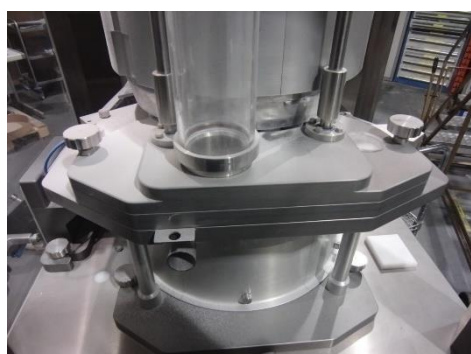
TPR 200 after 8 hours production before cleaning
