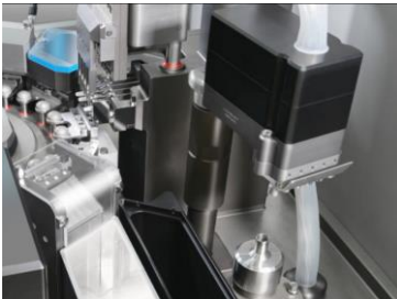
Integrated balance for fully automated In-process control (IPC)
