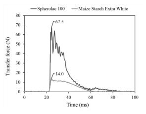
Transfer forces of two excipients, maize starch and lactose. One shows a significantly higher transfer force. In both experiments, the same process parameter settings were used.
