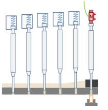
Schematic of the transfer force measurement. With this option, transfer forces can be measured in both directions: Positive force needed to push the powder plug out of the dosing disk and negative force to pull the pin back into its upper position.
