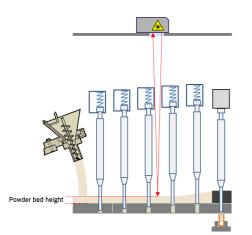
Schematic of the laser measurement of powder bed height. Delivers the possibility to directly monitor the powder bed height.
