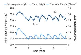
An example of the influence of powder bed height. In this special application (low powder bed height, bad flowing product) the powder bed level needs to be controlled accurately to ensure a good filling process.
