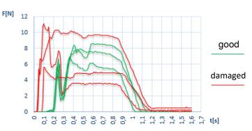
Different measured closing forces. Green: Capsules with no defect. Red: Capsules with closing defect.
